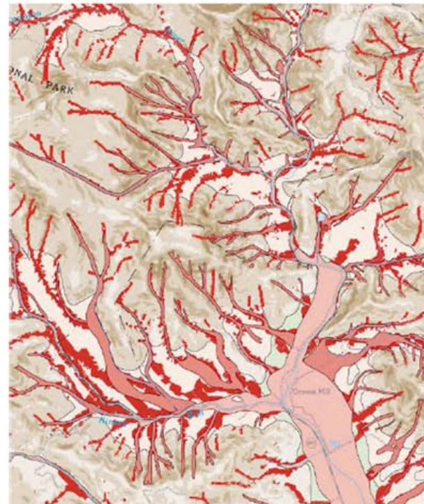
Fig. 28. Debris flows generally follow the drainage. The mapped area experienced debris flows and flooding during a large storm on June 27, 1995, in Madison County, Virginia. This debris-flow hazard map shows historical and potential debris flow and flood areas for that region.
