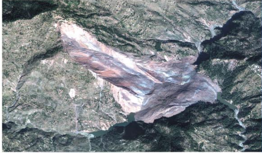
Satellite view of landslide dam caused by 2005 Kashmir earthquake (magnitude 7.6).
