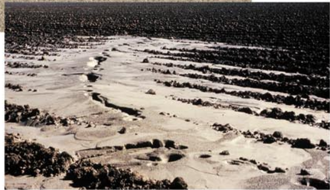
Fig. 18. When the underlying sand layer liquefied during the 1989 Loma Prieta, California, earthquake (magnitude 6.9), sand boils erupted along a ground crack.
