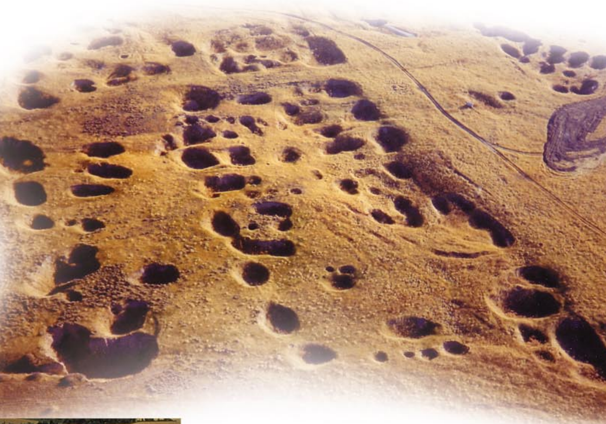
Fig. 34. Aerial view of subsidence pits above an abandoned underground coal mine in the Powder River Basin of Colorado. Collapse is occurring above "rooms" in the mine where coal was removed. Areas that have not collapsed are above the pillars of coal the miners left to provide support. Note the dirt road for scale.
